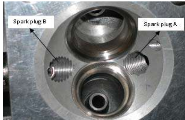
Details of spark positions in a DTS-i engine [3] .
